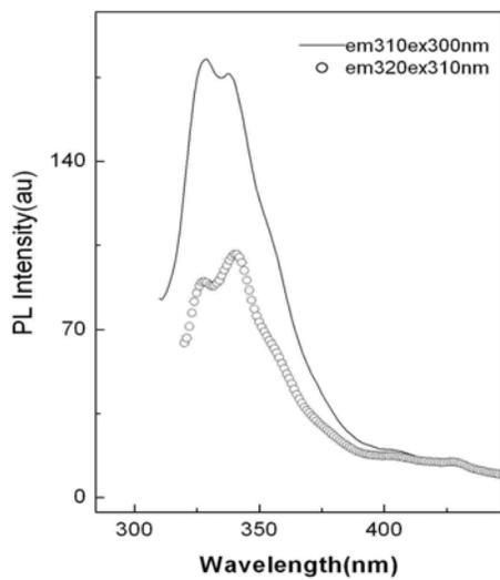
Fig.5: PL-spectra NiO nanoparticles at excitation wavelength 300nm and 310nm
