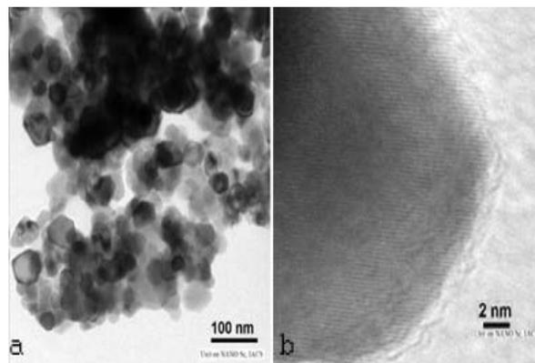
Fig.2: (a) Typical TEM image of NiO nanoparticles, (b) HRTEM image of NiO nanoparticles showing the fringe pattern of NiO crystal
