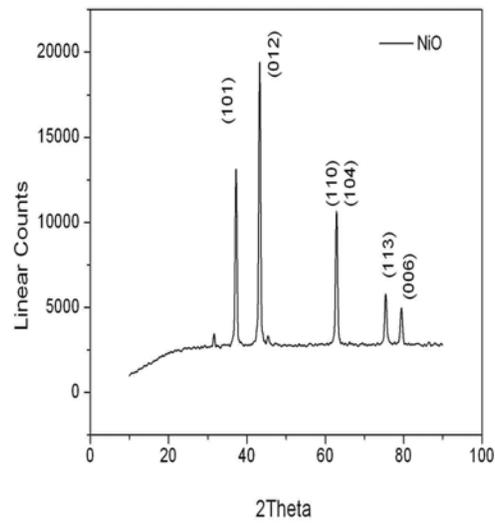
Fig.1: XRD pattern of NiO nanoparticles. Corresponding planes are indexed within the figure.
