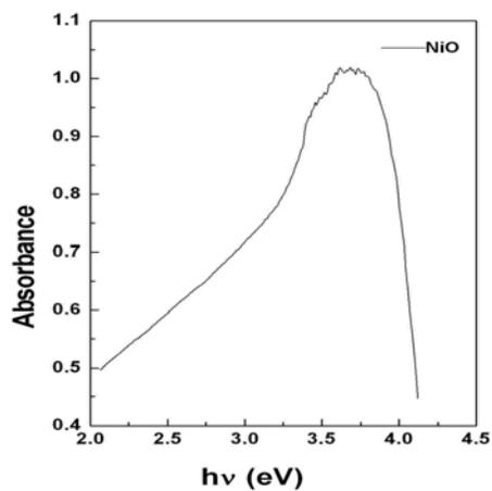
Fig.4: UV-Vis absorbance curve of NiO nanoparticles
