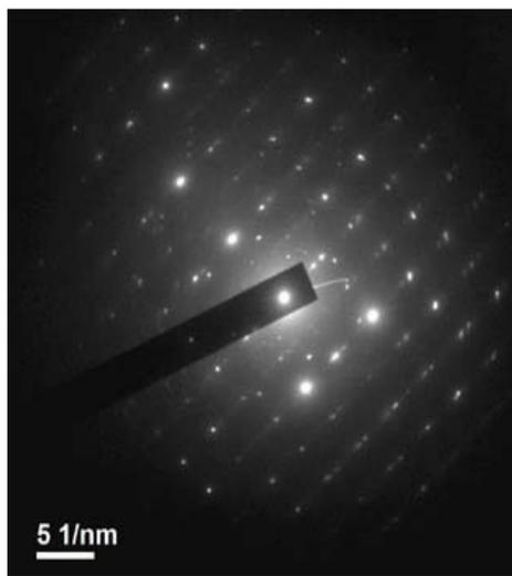
Fig.3: SAED pattern of NiO nanoparticles taken from the sample position shown in Fig. 2(b)
