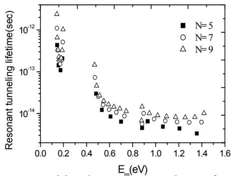
the ones with other values of resonant energies in the same band. As the band gap is proportional to the barrier height and the group velocity is inversely proportional to the bandgap, RTL always assumes higher values for larger  $y$ . So, an increase in the mole fraction accompanies a decrease in the peak width of the transmission spectrum at the resonant level of the superlattice.
