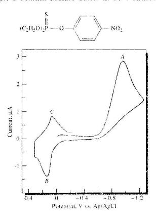
Using the observed cyclic voltammogram confirm the product produced at A, B and C position.
