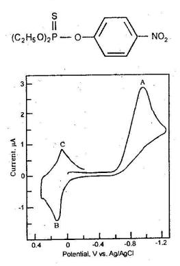
Explain the observed cyclic voltammogram confirming the product produced at A, B and C position.
