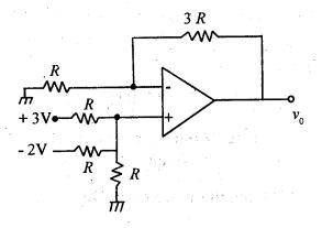
(h) Find the high frequency input impedance of the following op-amp circuit.
