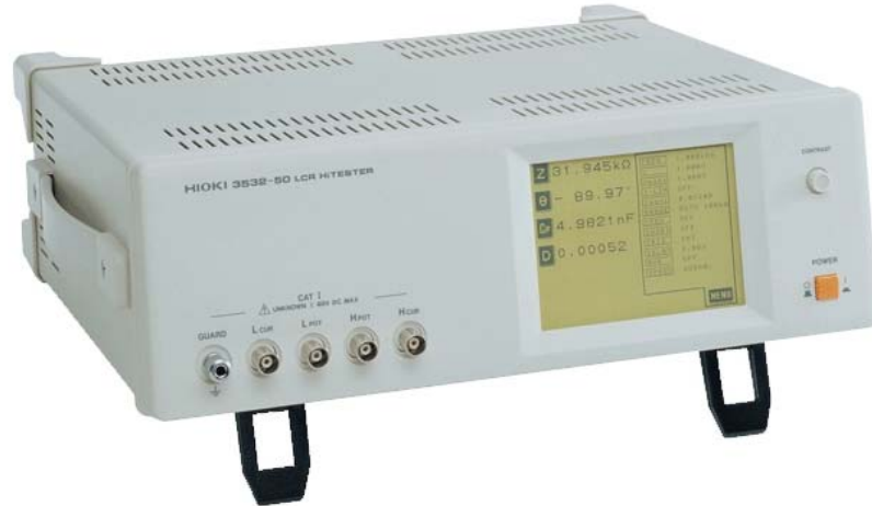
Fig. 3.7. LCR meter (HIOKI 3532-50 LCR HiTESTER, Japan) (Magnetism and Magnetic Material Laboratory, IIT Kgaragpur, West Bengal).
