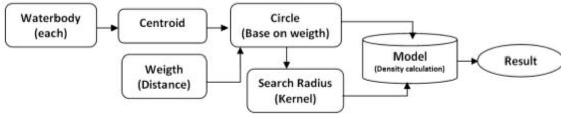
Figure 4.1 Workflow diagram of water density (KD) estimation
