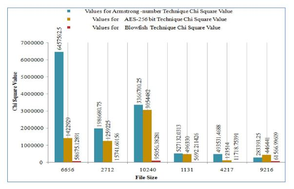
Figure 5.14: Comparison between APCS Algorithm, AES and Blowfish Algorithm in respect of Chi-Square value
