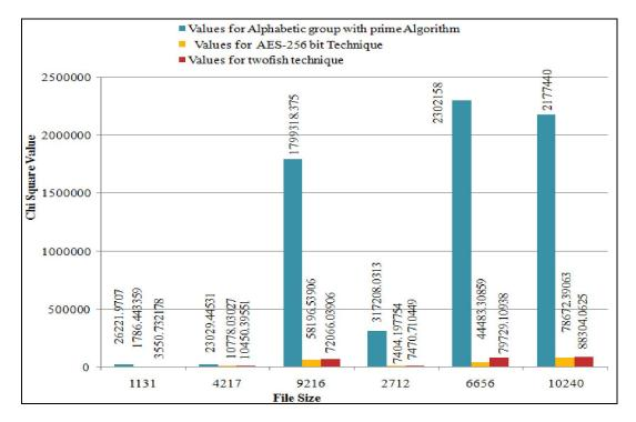
Figure 5.4: Comparison between PAG Algorithm, AES and Twofish Algorithm in respect of Chi-Square value
