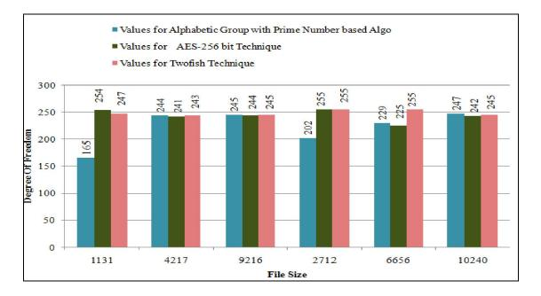
Figure 5.5: Comparison between PAG Algorithm, AES and Twofish Algorithm in respect of Degree of Freedom
