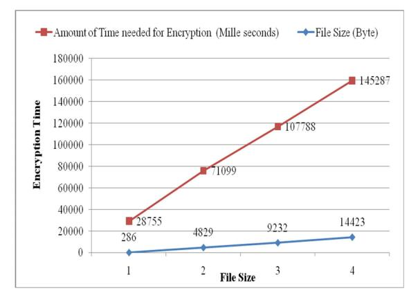
Figure 5.8: Graphical Representation of the Relationship between Encryption Time and File Size
