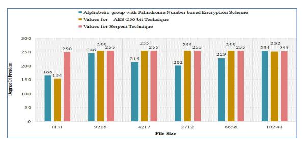
Figure 5.10: Comparison between PAGO Algorithm, AES and Serpent Algorithm in respect of Degree of Freedom
