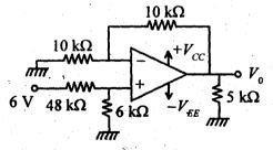
Find out the output voltage  $V_0$ .
