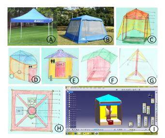
**Fig 5**: Utility and form generation exercises. (A) and (B) act as inspiration, where (C), (D), (E), (F) and (G) are the form explorations; (H) is the functional layout of different components and (I) is CAD exploration.
